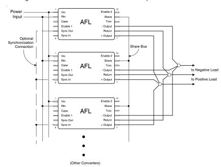
Figure III. Preferred Connection for Parallel Operation
