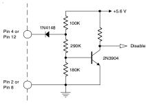
Internally, these ports differ slightly in their function. In use, a low on Enable 1 completely shuts down all circuits in the converter, while a low on Enable 2 shuts down the secondary side while altering the controller duty cycle to near zero. Externally, the use of either port is transparent to the user save for minor differences in idle current. (See specification table).
